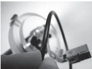
Take the time to inspect the O-ring on the canister lid before every dive. The O-ring should be free of grit or dirt and should not have any signs of damage. Remove the O-ring from the lid and wipe it down with a clean cloth before every dive. The O-ring groove on the lid should also be cleaned of any dirt or debris.
