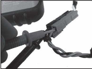
*To test the NiMH battery pack, your volt meter must have long enough probes to reach the middle of the connector assembly.*
